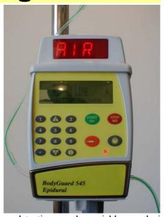
air-in-line detection and variable occlusion pressure settings, bolus delivery rate & infusion rate limiter.
